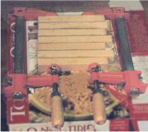
Glueup of a two-dimensional-pattern piece in pine & cherry veneer
