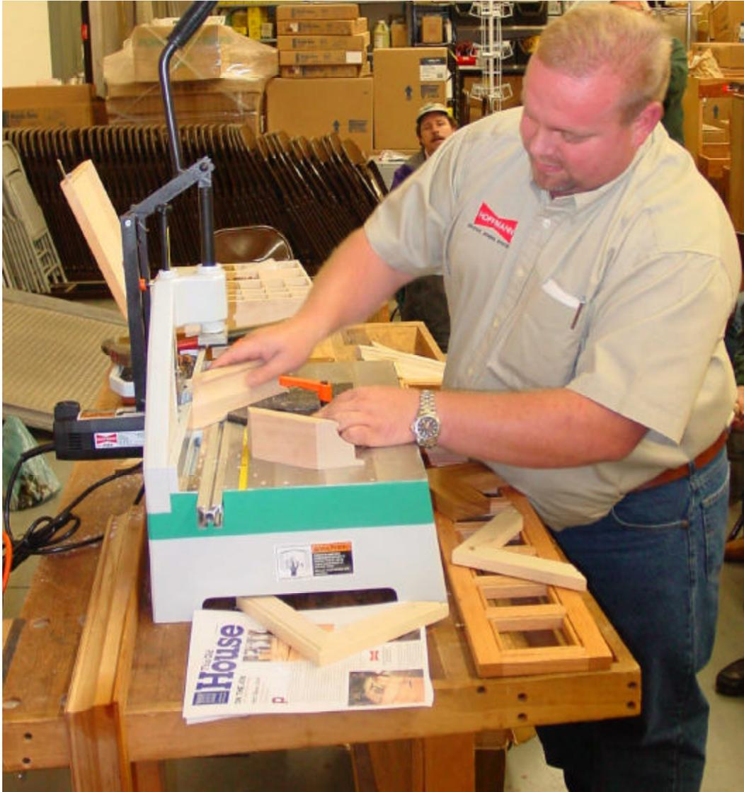
Gary demos method to join crown molding using the MU2
