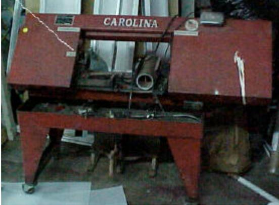
Vertical/ horizontal metal cutting bandsaw with 8" cutting depth by Carolina of Traveler's Rest, SC. Saw has a new motor with less than 10 hours of use. Blade is 115 1/2" by 3/4". The unit is 41" high and 51" wide. Will sell for \$500.00.
