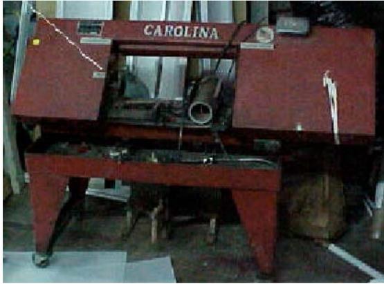
Vertical/Horizontal metal cutting bandsaw with 80" cutting depth by Carolina of Traveler's Rest, SC. Saw has a new motor with less than 10 hours of use. Blade is 115 1/2" x 3/4". The unit is 41" tall and 51" wide. Will sell for \$500.00.
