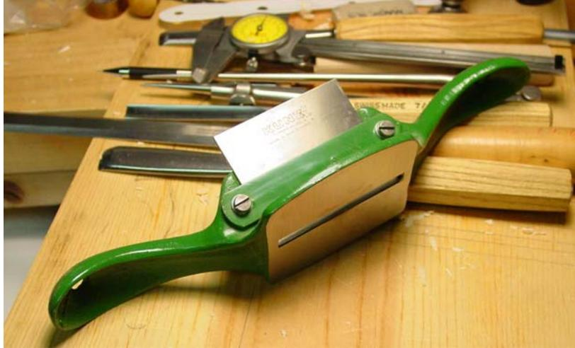
Figure 2 - an Example of a Cabinet Scraper
