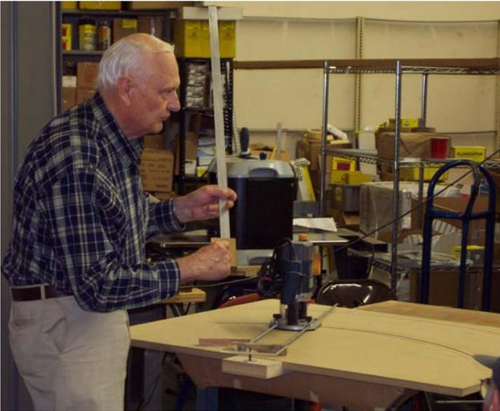
**Ralph continues to show us the various stages of use for the half-circle jig. Here he has made several trammel-type devices to cut the inside and outside of a curve.**
