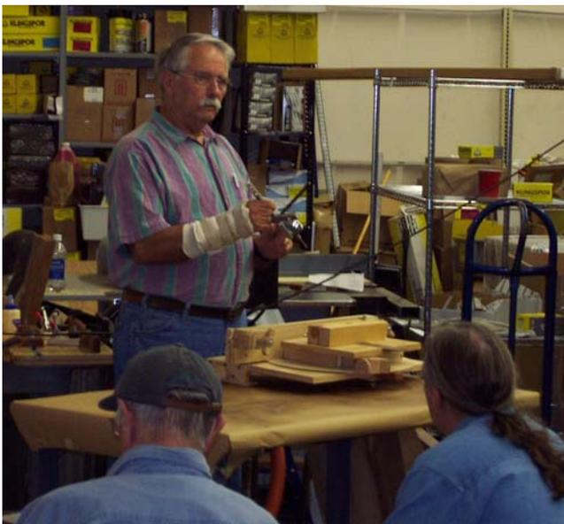
**In George's hand is a simple jig to check the alignment of your table saw blade to the miter gauge slot.**
