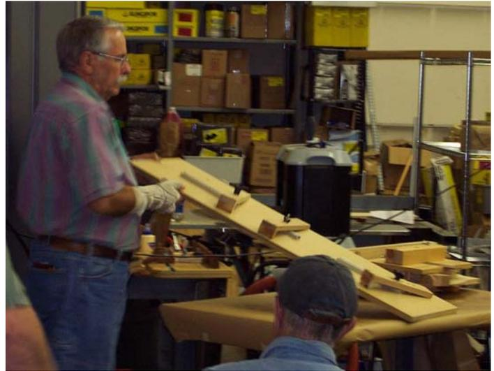
**This jig, George had not used yet, is used to clamp up cabinet doors, as well as other things. This jig allows for varying width pieces and includes built in cams to tighten down the piece. This jig also helps keep a good 90 degree joint!**
