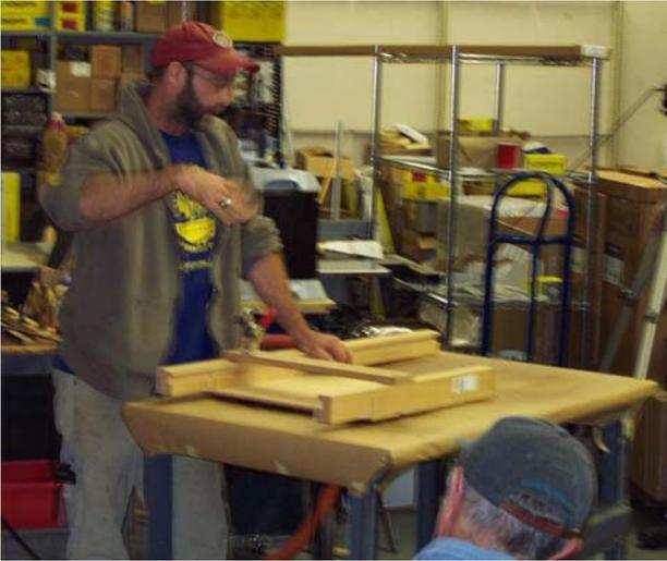
**A crosscut jig for the table saw or bandsaw.**
