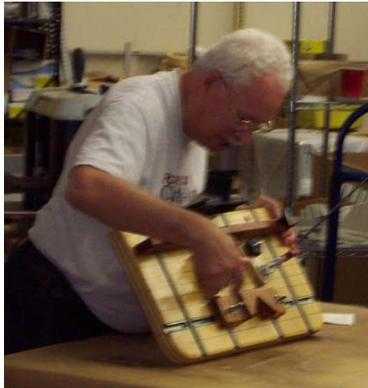
**This jig is an auxiliary table for Bill's Shopsmith, this allows him to mount up a PC RO spindle sander.**
