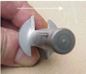
*Turn the router bit-end-down and things change. The arrow shows bit direction in this mode. The stock, using the top edge of the bit, would have to be fed right to left.*
