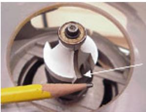
*The pencil is aimed in the direction the bit turns, the arrow shows the feed direction. Seeing the cutting edge makes figuring this feed direction easy.*
