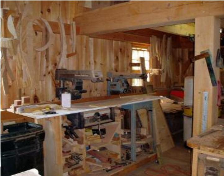
As you enter against the left wall I have the two radial arm saws stationed. The saws share a common table and are mounted on a common base with casters. The cutoff table is 8' in length. The right saw is dedicated for crosscutting, and the left saw is equipped with a dado blade for cutting joinery. There are bins beneath for cutoffs, and a large scrap container on the left end for waste materials.
