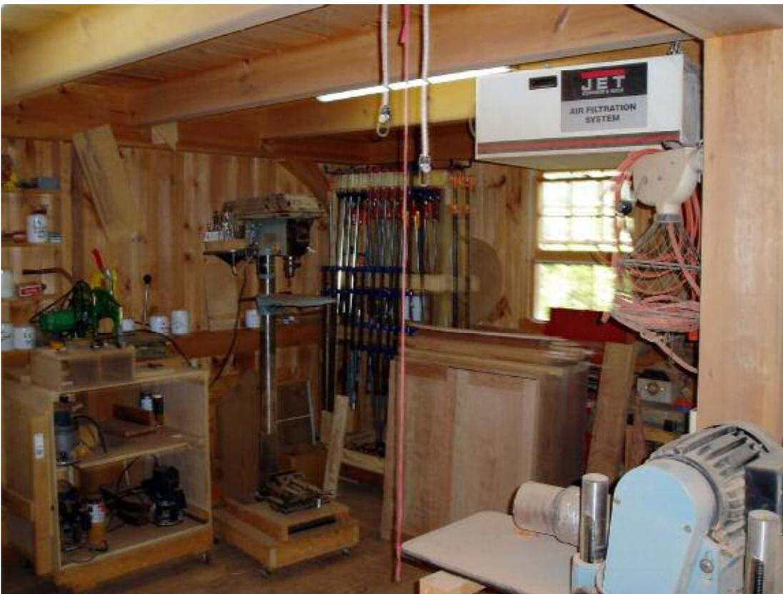
The drill press is located in the far right corner with a clamp rack against the near wall. Both of these incorporate mobile bases as well. Just barely visible on the far right is the drum sander. Though the drum sander is not used very often and takes up needed floor space I'm not quite ready to part with it yet.
