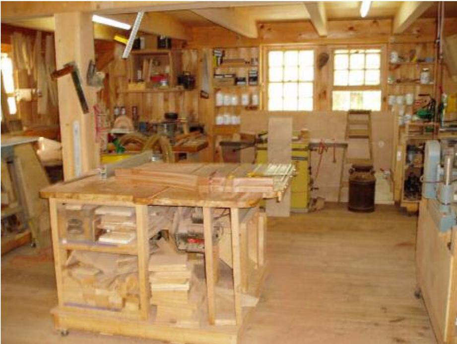
As you enter the shop you will see that the table saw is located in the center. This allows me to rip exceptionally long material (12' +) by opening the front doors. The planer is located to the right of saw that long material can be planed as well.
