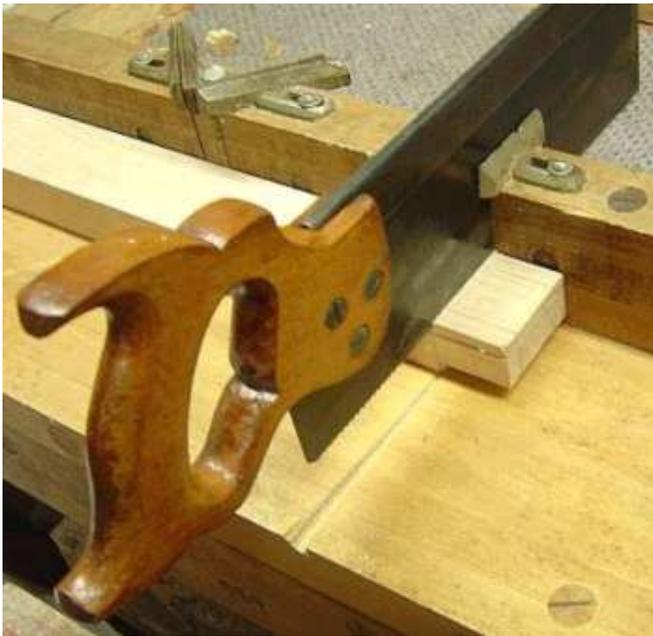
When using handsaws, tilting the workpiece away from you and beginning at a corner is the most efficient technique for hitting the outside edge of those lines on the first try.
