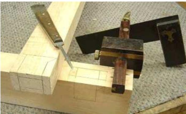
This is a 6/4 by 3" post and a 5/4 by 2" rail, and I'll do a 3/4 by 1 1/4" mortise (+ a 16<sup>th</sup> of an inch over) deep to house a 1 1/2" long tenon. Mortises should always be slightly over deep to allow room for glue squeeze out. A 7/8" wide mortise would also be acceptable here. The *haunch* is the 45° tenon stub I've drawn on the upper face profiles of the stock that increases the gluing surface and aids in the joint resisting twisting stress.
