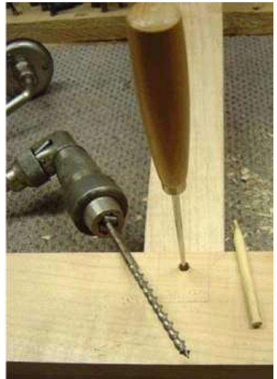
...then dry assemble the joint and use an ice pick from my lofting kit to mark the hole center on the tenon.
