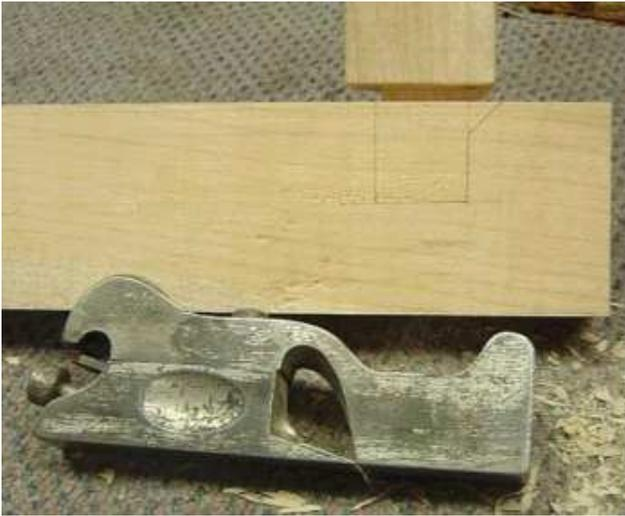
You can see from the relatively small pile of shavings that bringing the tenon from *won't fit* through *drive fit* to *snug*, *heel-of-the-palm*, *hand fit* didn't require much work. The edges of the tenon can be relatively loose compared to the tight cheeks, as chopping hard with that steep-beveled chisel has compressed the end grain at the ends of the mortise slightly...and they'll swell back some as the humidity increases.
