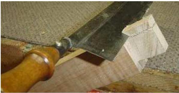
...and finish the miter using the dovetail saw. The more perfect my layout and saw cuts, the less plane work will be needed...but providing I remain outside those scribed lines, even my sloppiest cuts...and there are certainly some sloppy ones here...can be easily planed to perfection.
