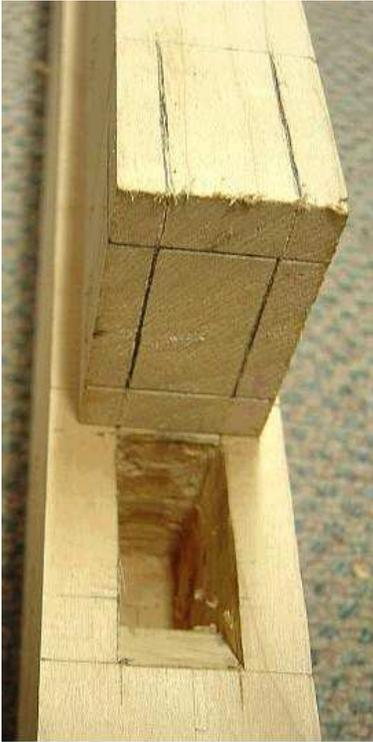
The end result is a clean, accurate mortise done in mere minutes. Depending on the size of the mortise...in average-sized furniture stock and using the right tools, they can be chopped at the rate of between 6 and 20 per hour with very little practice at it...on many pieces faster than the time needed to set up and test a router jig.
