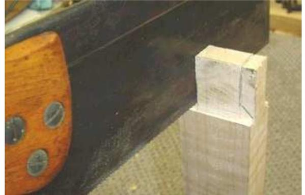
...rip the lower edge of the tenon and the unmitered section of the upper edge...
