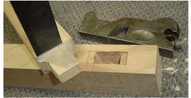
A technique I use on fine furniture I'm only demonstrating here is to pare the tenon shoulders inward from the edge slightly using a bench chisel. This insures a perfectly tight shoulder-post fit by removing any impediments in the tenon-shoulder corners.
