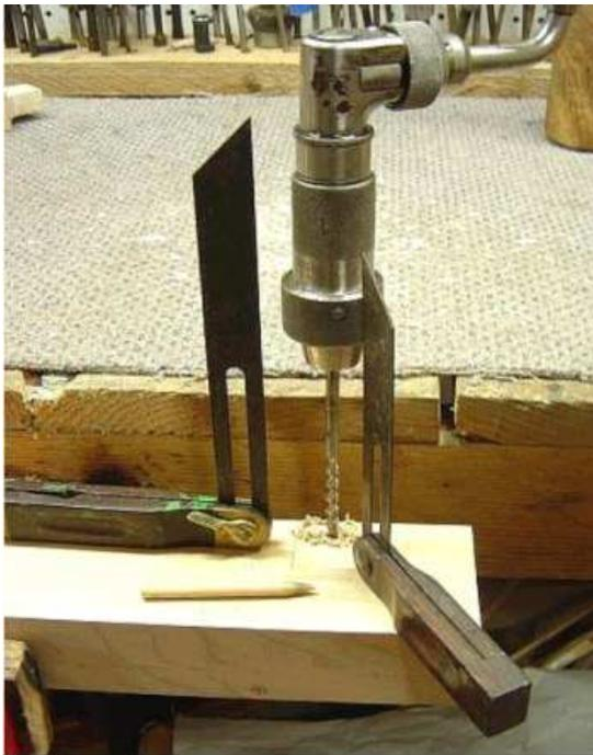
To make the drawbore, I simply point a dowel and drill a plumb hole to match through both mortise cheeks...
