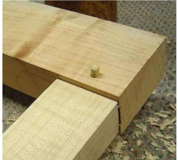
...and I prepare for final assembly. The post is cut to final length, glue is applied, the joint assembled, and that pointed peg driven through the offset holes which pulls those shoulders with considerable force against the post for a bulletproof structural joint that really needs no glue.
