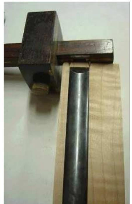
You can also see in the previous photo that if the rail is to be flush with the post top, then I've crosscut the post too long. You are correct, I have. The post's short grain on the topside of the mortise will be far too fragile to chop a mortise and haunch without pre-drilling...and pre-drilling is unnecessarily slow, so I'll chop my mortises vigorously and trim the tops of the posts later.
