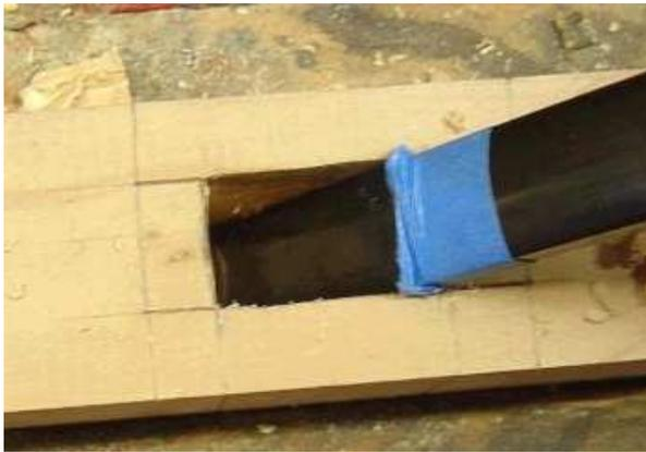
Upon reaching the correct depth, the mortise bottom is squared and cleaned by lightly striking the chisel with the bevel instead of the blade back indexed against the mortise end ...
