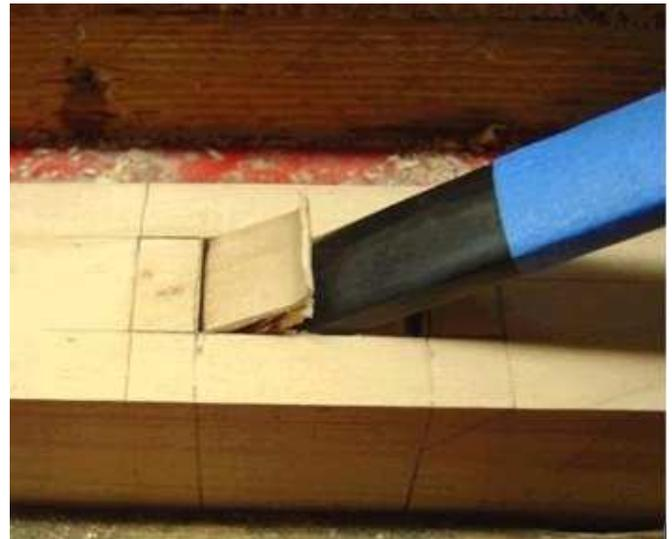
The third blow is taken bevel up about a third of the way along the mortise's length at an angle downward toward the end...
