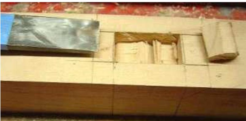
...as the mortise gets deeper, the obstruction of the mortise ends force the angled blows increasingly steeper, eventually preventing them from reaching within clean splitting distance from the end blows...the chisel is then flipped and the angled blows struck bevel down to keep the cutting angle sufficiently acute for clean, four-chop split outs.
