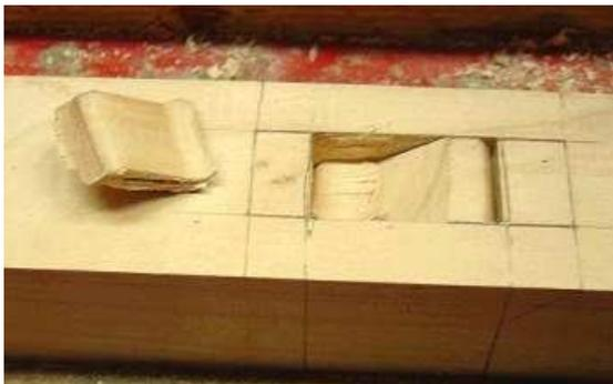
...and the waste levered out, splitting along the grain of the wood. The deep scribe marks from the mortise gage prevent any chip out.
