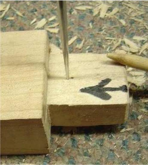
The joint is disassembled and the hole for the tenon bored a 16<sup>th</sup> or so *inboard* of the mark for the cheek holes toward the tenon shoulder...
