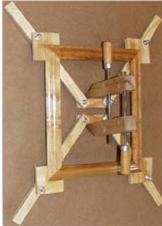
This simple jig is self-squaring and requires only one clamp to firmly secure the frame. When pressure is applied, the jig evenly distributes the pressure to the four corners. The "L-shaped" cleats prevent the frame pieces from sliding out of alignment. The jig pictured here will work for frames twice as large. 2-1/2" carriage bolts are used to hold all of the parts together. Larger or smaller frames can be clamped by drilling additional holes and moving the cleats.
